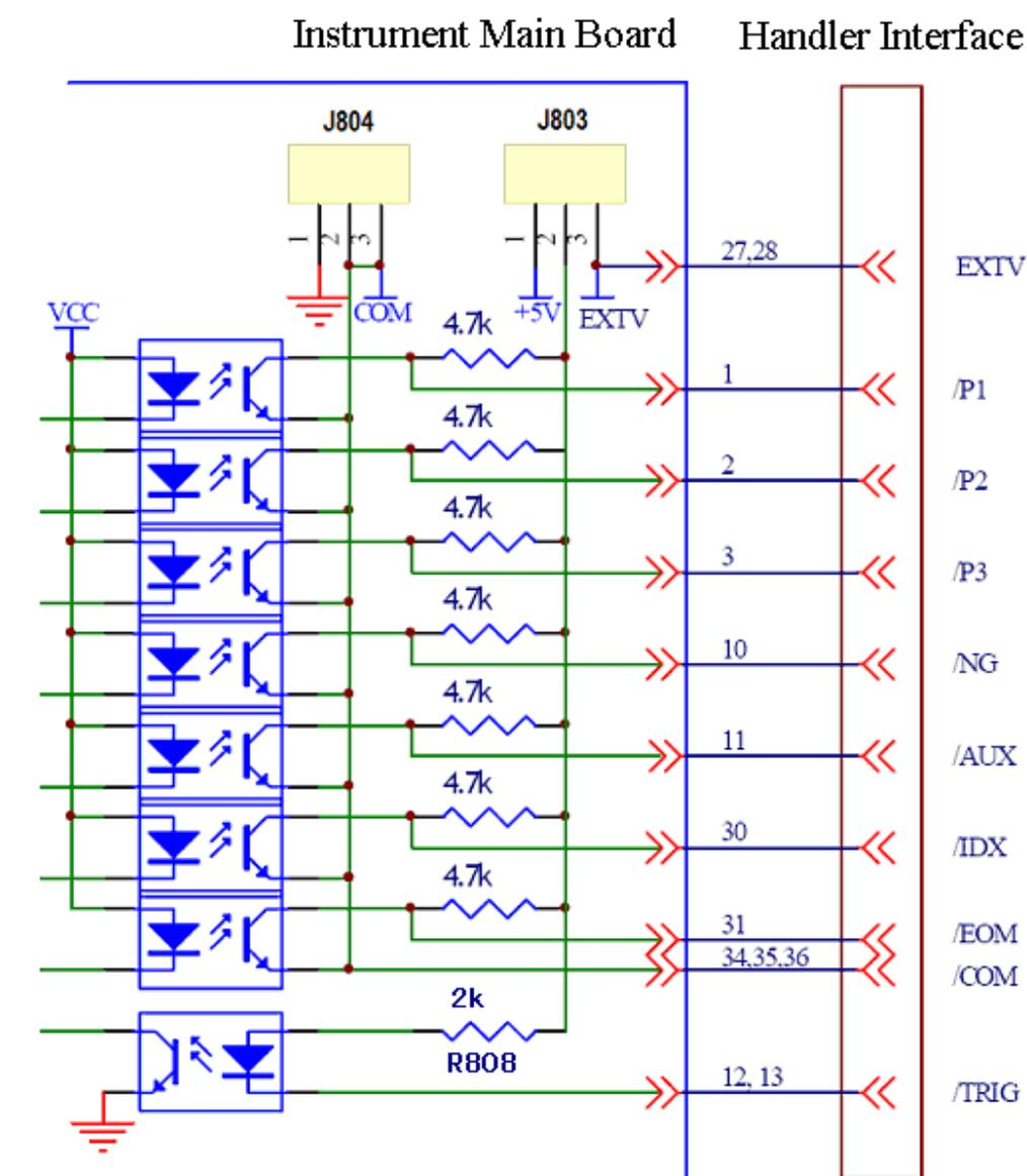
Fig. 6 – 4 Simplified Schematic Diagram of Sorting Signal
