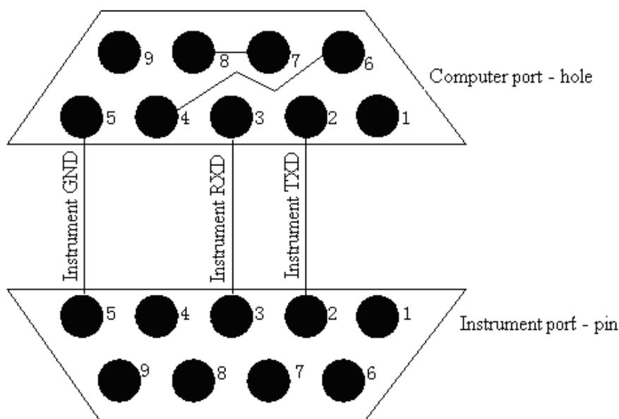
Pin 2: transmission port      Pin 3: Receive port      Pin 5: Ground (GND)
