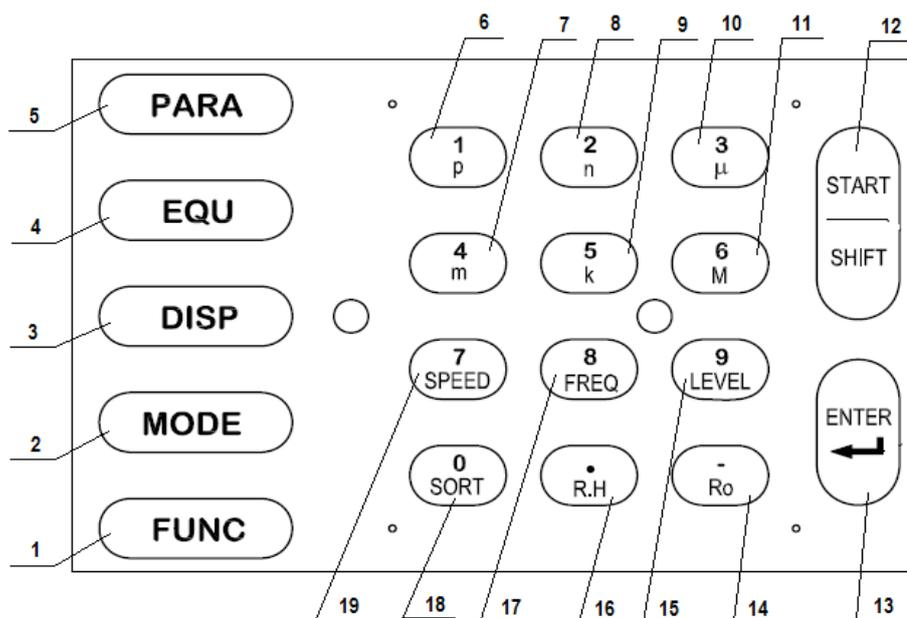
Fig. 4-2 Schematic Diagram of Model BR5810 Keyboard
